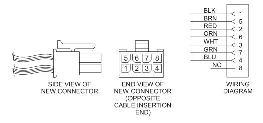
**NEW 8-PIN CABLE CONNECTOR (GUI END)**
