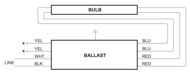
\* FOR SINGLE LAMP OPERATION, INSULATE YELLOW LEADS INDIVIDUALLY FOR 600 V
