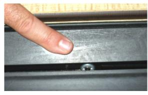
While there are no markings on the rail, the pinch points begin approximately 33" (838 mm) from the foul line end of the rail and exist at a point every 22" (559 mm). for the length of the rail.
