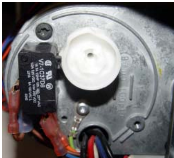
OLD MOTORS HAD TWO CAM ADJUSTMENTS FOR THE UP AND DOWN TIMING POSITIONS OF THE MOTOR
