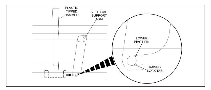
If you have recently replaced any support arms, check them to verify that they are installed properly. Failure to do this may result in broken vertical support arms.
