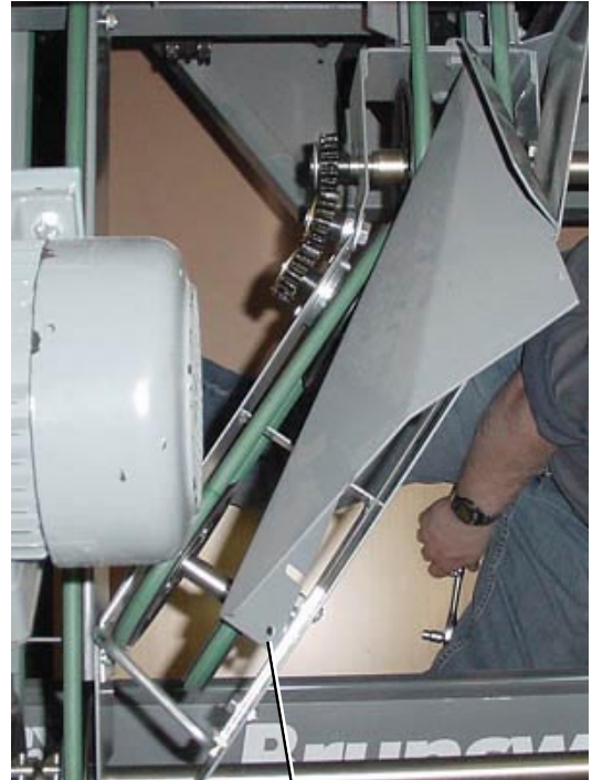
CORNER TURN PLATE REMOVED
