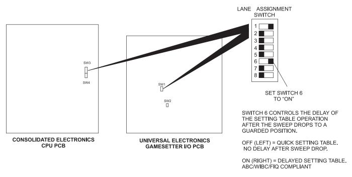
Additionally, centers that have pinsetters with consolidated electronics may, on occasion, experience a problem during a short cycle where the sweep is not raised to the up position. Setting switch 6 to the "on" position will typically correct this situation.
