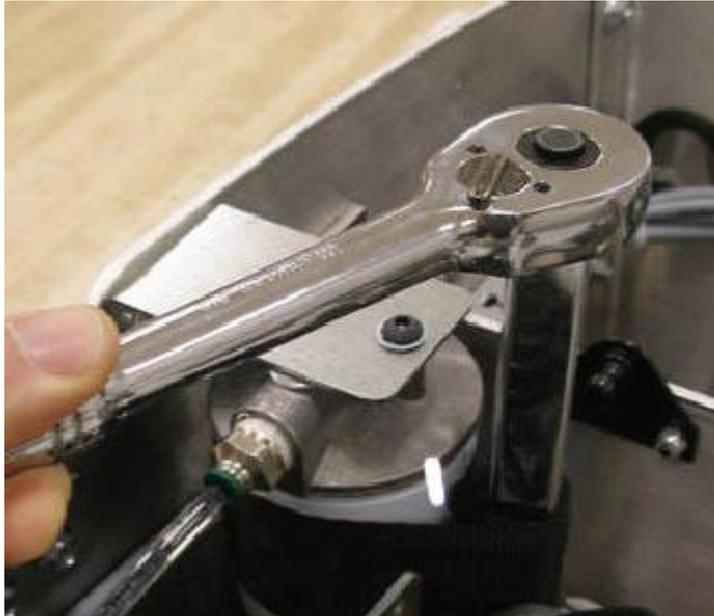
Tighten the Spin-On Oil Filter one full turn past the original mark. Use the filter wrench if needed. Refer to Figure 5-19.
