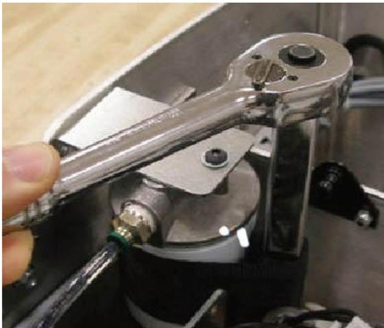
This should seal the filter to the housing at the correct point to prevent the filter from leaking during normal operation of the Authority22.
